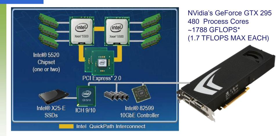
PCI Express 2.0 offers 4GB/s of peak bandwidth per direction for a x16 link and 8 GB/s concurrent bandwidth (duplex). ICH = I/O Control Hub  $_{Xeon 5500}$  (duplex).
