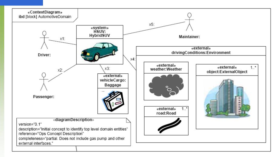
A System Context element is a virtual container that includes the entire system and its actors. Graphic courtesy of OMG SysML Modeling Language formal/2008-11-01
